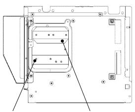
Reuse <u>the insulating sheet</u>. Applying thermal grease to the back of the insulating sheet makes it easy to attach the insulation sheet. Reuse <u>the sub heat sink.</u> Applying thermal grease to the surface and the back of the sub heat sink.
